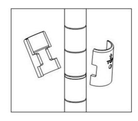
Note: There will be a very small gap in-between two locked SLIP SLEEVES (D)—this is normal.
